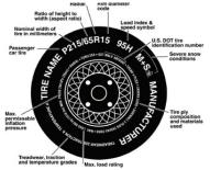
**P:** The "P" indicates the tire is for passenger vehicles. **LT**: The "LT" indicates the tire is for light trucks or trailers **ST:** An "ST" is an indication the tire is for trailer use only.
