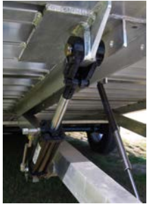
Hydraulic damper and gas spring for controlled lift
